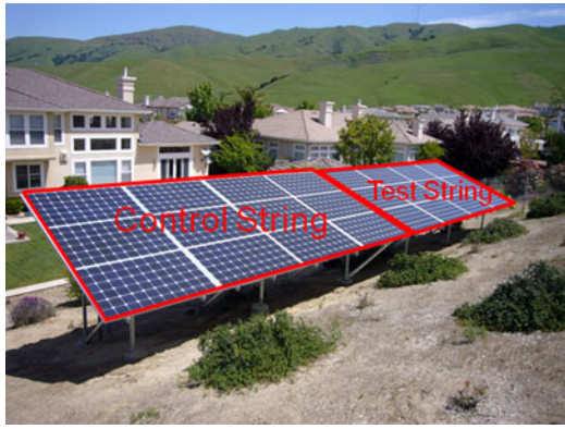
Fig. 19. 5.4-kW field test setup: 12 panels each in control string and test string.
